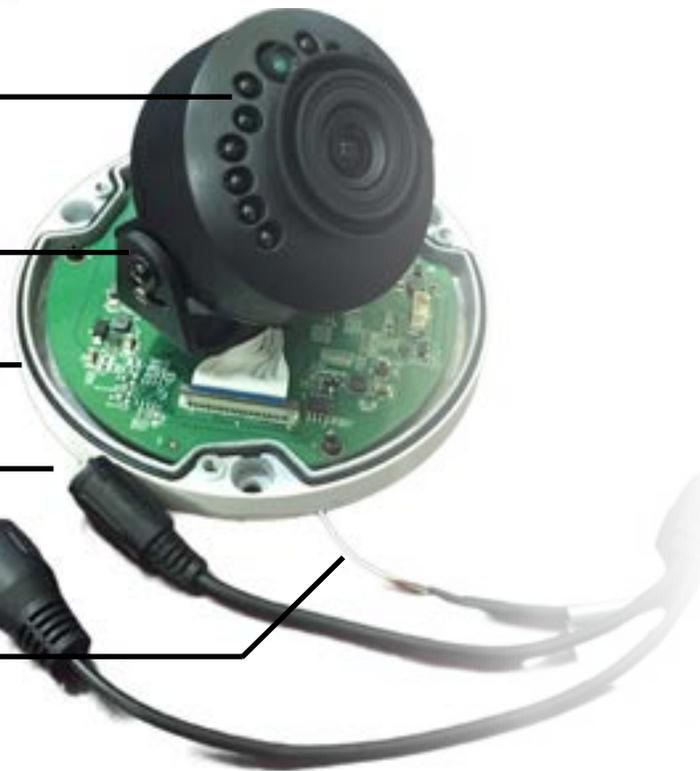
When the Standard definition/high definition switch control cable is short circuit, systems outputs standard definition video. Otherwise, when the circuit is open, system outputs the high definition video.
